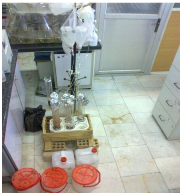
(Fig. 3): A view of Column leaching equipment
