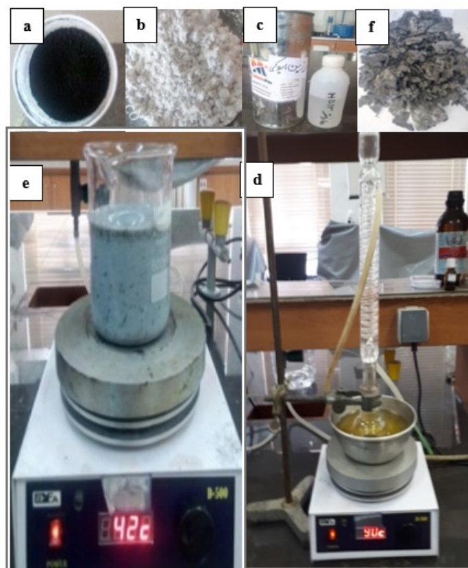
Fig. 1 PCD production process (a) carbon nanofiber (b) diatomite soil (c) Epoxy resin and hardener (d) thermal reflux system for polymeric composite (e) adding achieved suspension to deionized water (f) produced PCD sample.
