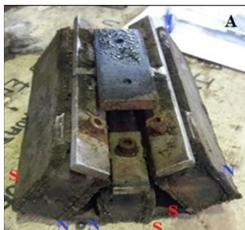
Figure 2: Depictions of the magnets and position of the N and S poles (A) and a schematic diagram of the pulp moving in a separator (B)
