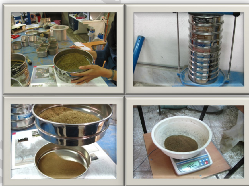
Fig. 2. Sieve analysis equipment used for different polluted horse bedding
