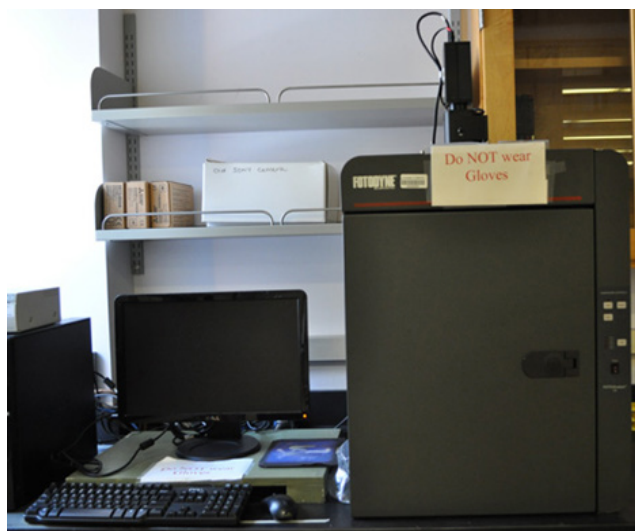
Fig. 10. Gel documentation system for observing stained bands on gel [11].
