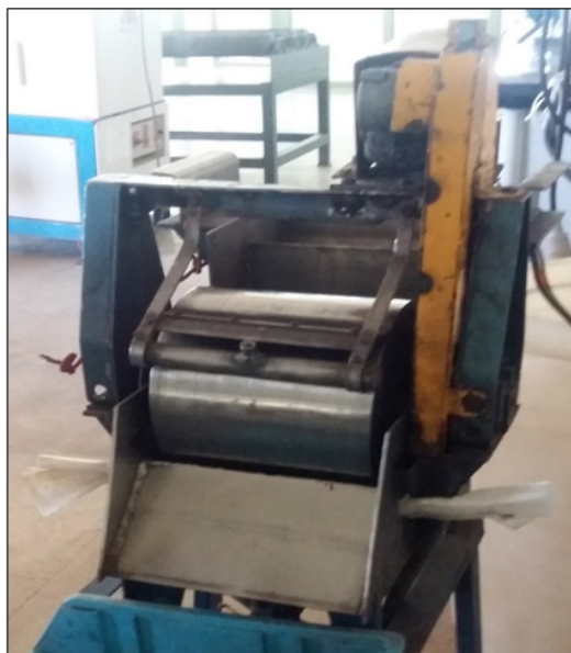
Figure 1: View of the wet low intensity magnetic separator device (BOXMAG-Rapid model)
