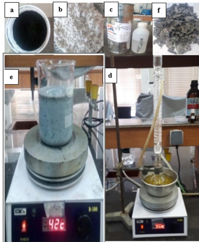
Fig. 1 PCD production process (a) carbon nanofiber (b) diatomic soil (c) Epoxy resin and hardener (d) thermal reflex system for polymeric composite (e) adding achieved suspension to deionized water (f) produced PCD sample.
